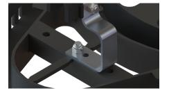
STEP 4. Fit the previously assembled support bracket through the top of the screw and secure it with a lock nut using a 1/2" wrench. Repeat the process for the second support bracket.
