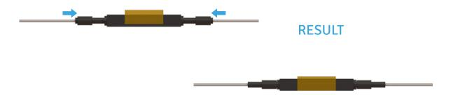
1.9 Press the yellow part until it stops to splice the fibers and to finish this process.
