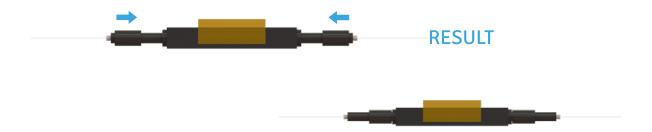
1.8 Press the yellow part until it stops to splice the fibers and to finish this process.
