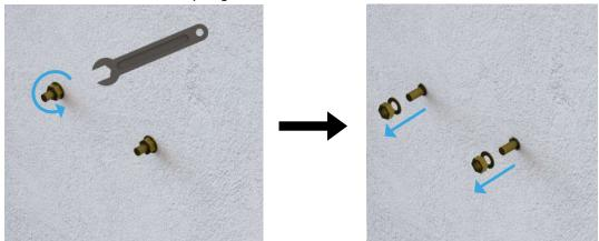
Align the multiport service terminal installation hole with the screw M8x1.0. Insert again the spring washer and the nut M8 in that order.
