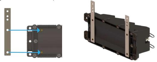
Insert the flat screws M5 X 0.8 fixing the metal holders to the base of the Multiport Service Terminal using a phillip screwdriver.
