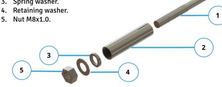
Using a drill and concrete bits make the blast-holes on the wall for the 4 Multiport Service Terminal installation holes according with the standardized measures of concrete bits corresponding to the screw M8x1.0.
