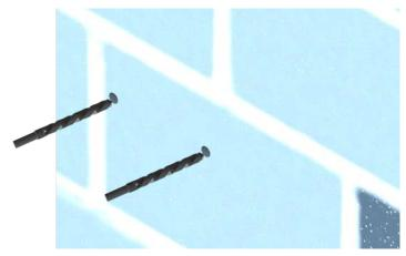
It is recommendable to make the blast-holes using a 6.5mm [1/4] bit as a guide then the 8mm [5/16] bit.
