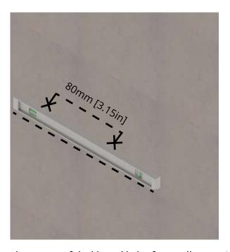
The distance between the centers of the blasted holes for a wall mount installation is 80mm [3.15"]
