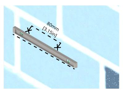
The distance between the centers of the blasted holes for a wall mount installation is 80mm [3.15"].
