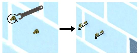
Align the multiport service terminal installation hole with the free part of the screw M8x1.0. Insert again the spring washer and the nut M8 in that order.
