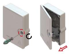
Fig. 1 Opening of the terminal box.
