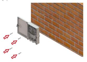
Fig. 3 Placement of screws and dowels.
