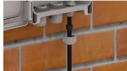
**Fig. 6** Cable passed through the parts of the input port.
