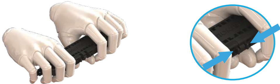
Closed splice closure
