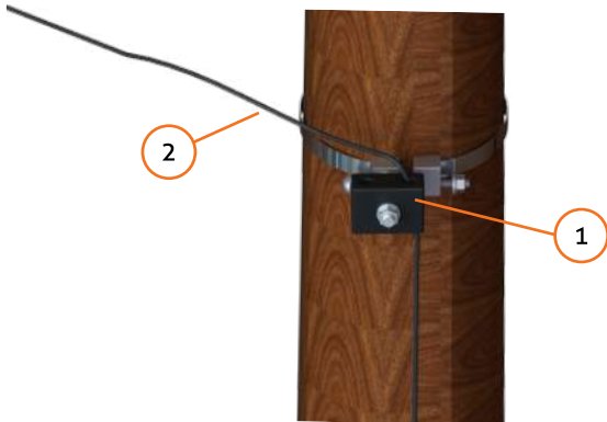
Fig. 1 Download clamp application on wooden pole
