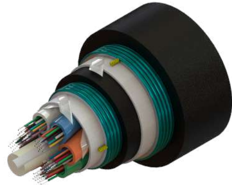
LOOSE TUBE DOUBLE-ARMORED DOUBLE-JACKET CABLE DRY 72F G652.D FIBER FT
