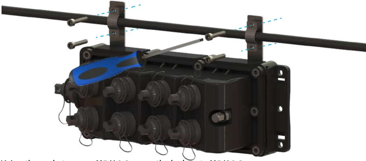
Using the socket screws M5 X 0.8 screw the lock-nuts M5 X 0.8. For this part of the process can be used a socket screwdriver or an adjustable spanner.
