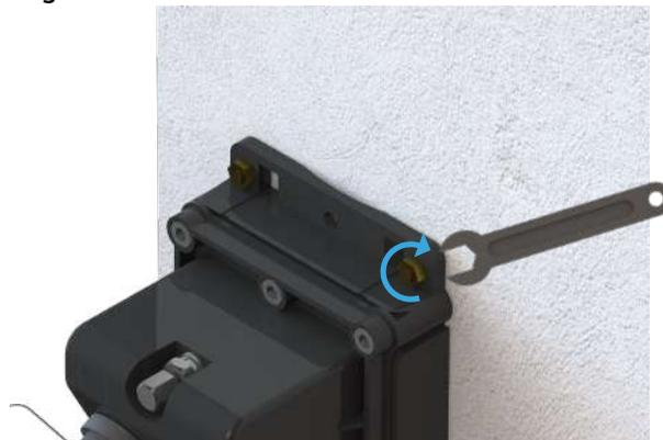
Note: Use a ratchet wrench or an adjustable spanner to fix or release the nuts.
