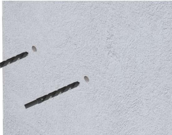
It is recommendable to make the blast-holes using a 6.5mm [1/4"] and a 8mm [5/16"] bits.
