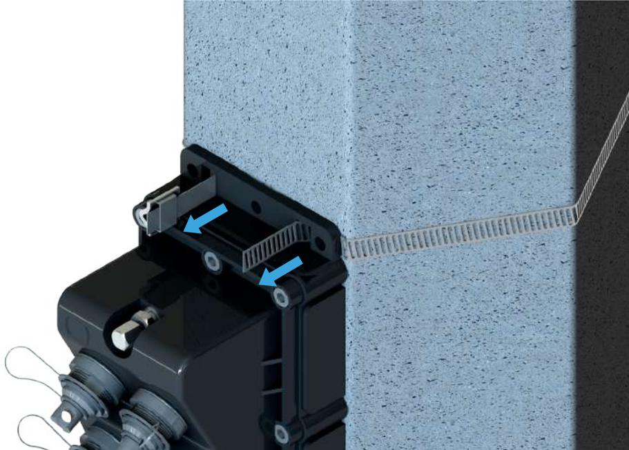
Insert again the tip on the suggestion clamp and using the flat-head screwdriver fix the metallic brace to the pole.
